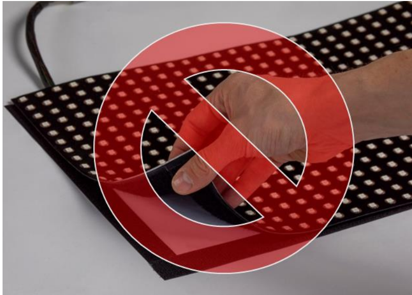
Figure 2: Excessive bending of ledTec.flex banner must be avoided
